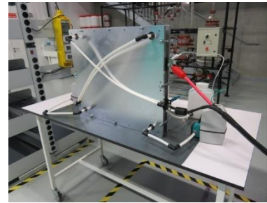
Industrial stack 4 kW prototype
